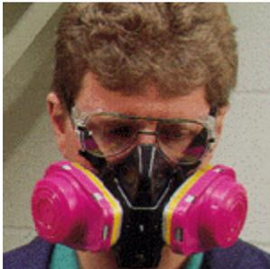
Combination respirator cartridges are normally used in atmospheres that contain hazards of both particulate and gases or vapors. They have particulate filters and gas/vapor cartridges combined. Specific chemicals must be known. An established change out-schedule must be established for these cartridges unless an end-of-service indicator is provided on the cartridge.
